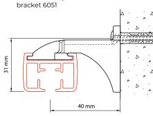
Wall mounting with adjustable extension bracket 6017, can be shortened from 15 to 7 cm.
