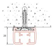
Concealed mounting on or in a ceiling with bracket 6055-3100-N-040
