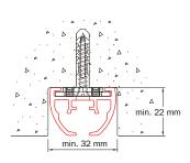
Mounting: turn & click into place Wall mounting with adjustable extension bracket 6017
