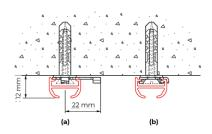
ceiling mounting 4600 with ceiling mounting clamp 2650 + washer, before (a) and after (b) fastening the ceiling mounting clamp
